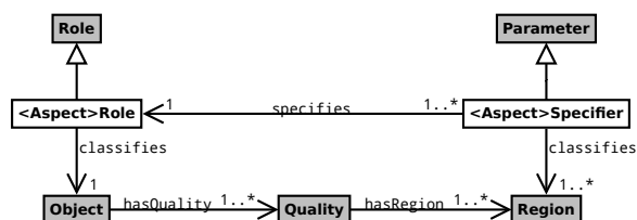
Fig. 3. Basic structure of a communication aspect in the Flow Control Rule Pattern. <Aspect> is a placeholder for Sender, Receiver, Content, and Channel.
